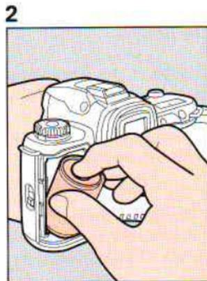
1. To open the back cover, slide the back cover release lever in the direction of the arrow.
